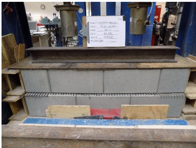
Figure 6 – Neoprene Pads, Loading Plates, and Beam
