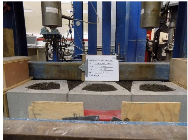
Figure 3 – First Course with Compacted Aggregate
