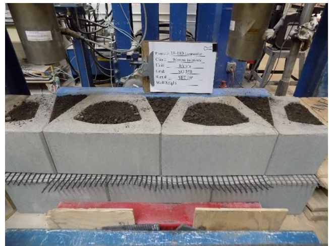
Figure 5 – Second Course of SRW Units with Aggregate
