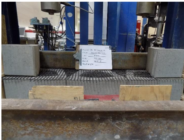
Figure 4 – Placement of Geosynthetic
