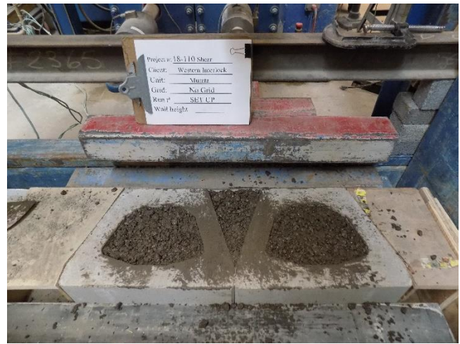
Figure 3 – Bottom Course with Compacted Aggregate
