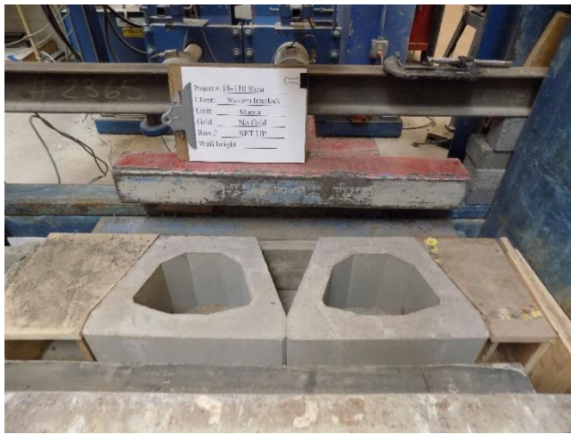
Figure 2 – Bottom Course of SRW Units
