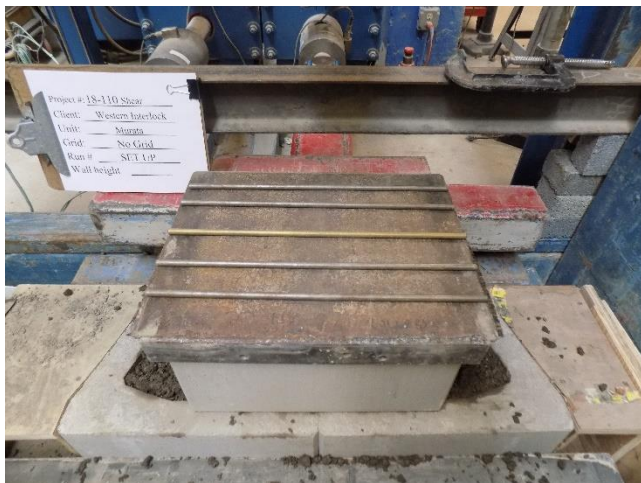
Figure 6 – Neoprene Pads, Loading Plates, and Beam
