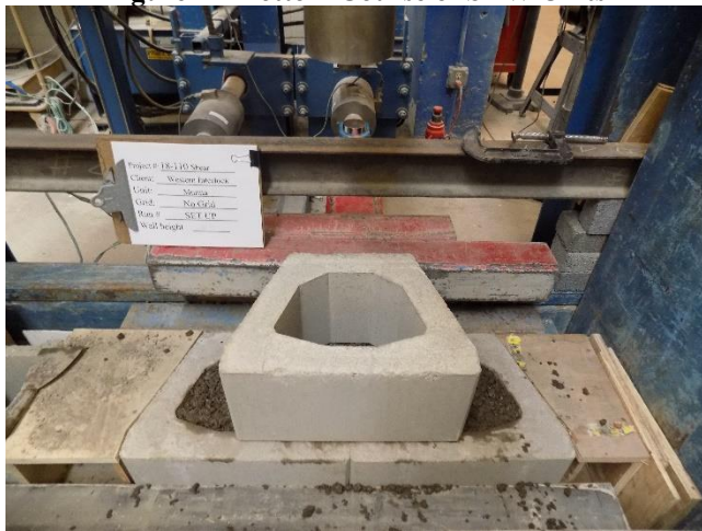
Figure 4 – Top SRW unit placed
