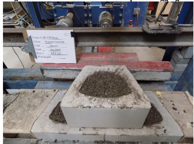
Figure 5 – Top course with Aggregate
